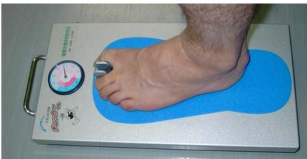
Figure 1 The device of toe-gap force measurement
