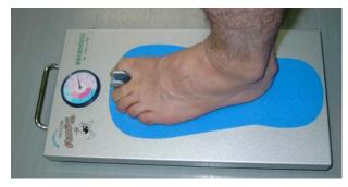
Figure 1 The device of toe-gap force measurement
